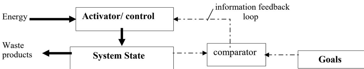
**Figure 8:** The basic feedback control process. The second law of thermodynamics requires energy input and heat output in active processes, which must occur then in an open system.
